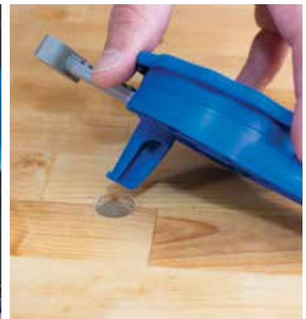
Works on any bench with 19mm bench dog holes—or drill your own.
