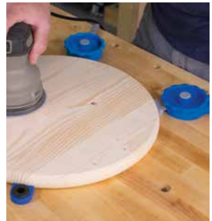
Clamp shoe holds flat and rounded shapes, as well as 90°.
