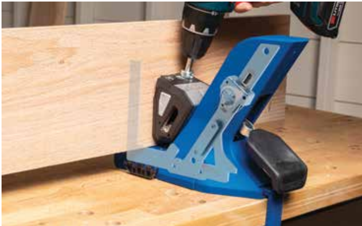
Multi-featured jig for creating pocket-hole joints in materials from 13-38mm thick
